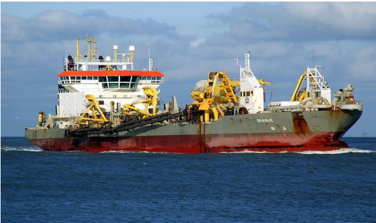
Image 8.9 Dredging Vessel (ORANJE Dredger) (Source: Wikimedia Commons)
