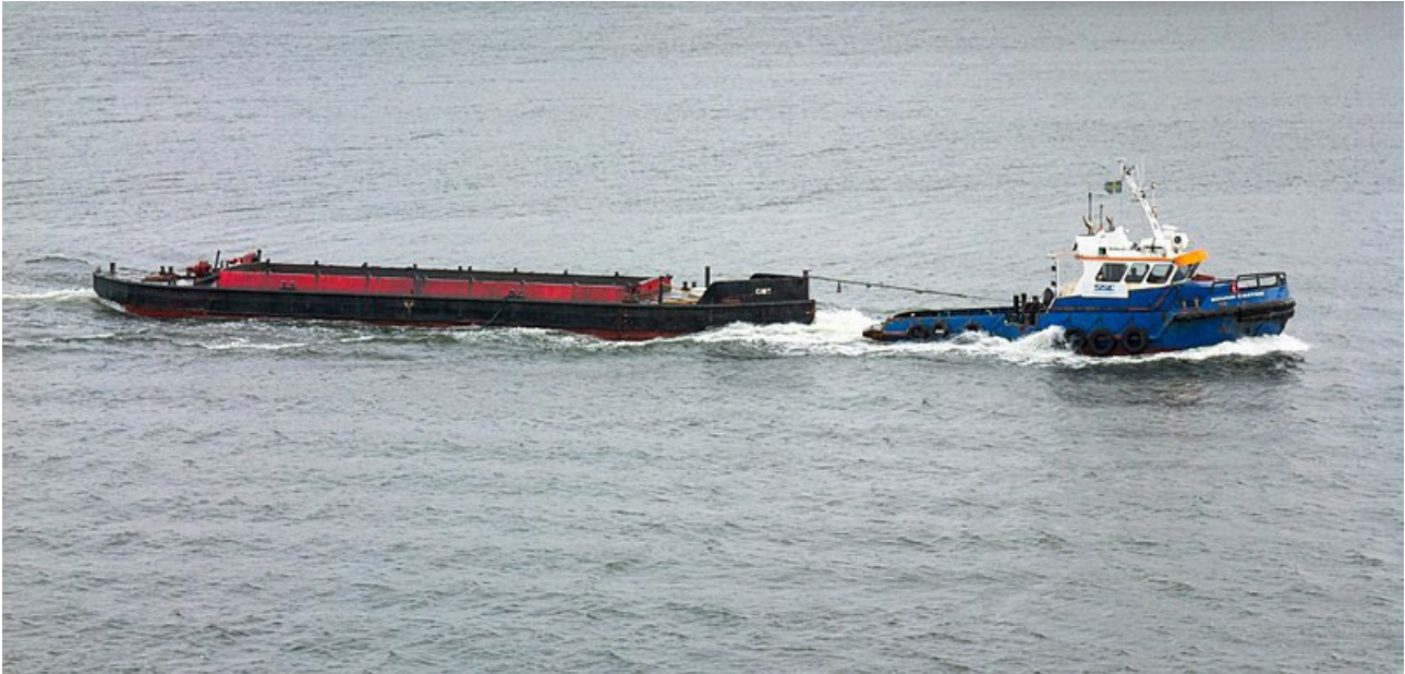
Image 8.8 Towing Barge (Sound Castor) (Source: Wikimedia Commons)
